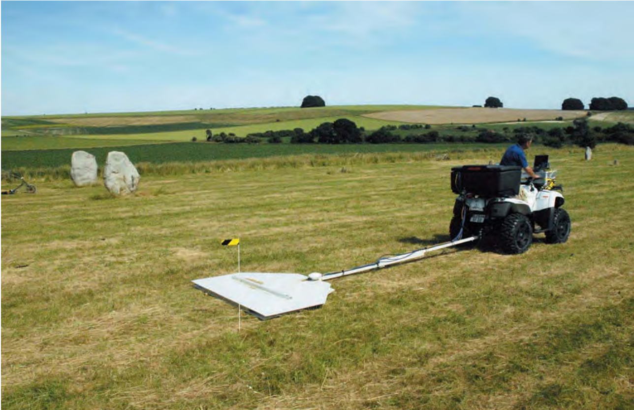
Plate 3 AMOS electromagnetic survey at in the West Kennet Avenue, Avebury, July 2013 (Photograph by Timothy Darvill. Copyright Reserved: BU, DAI and Sensys)
